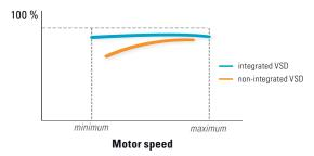
Special attention is given to the electric motor, which is specifically designed for VSD operation (inverter duty motor). Bearings are protected against induced bearing currents and both motor and converter are perfectly tuned to obtain the highest possible efficiency over the entire speed range.
