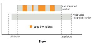
• The machine is tested for the complete speed range to eliminate any 'speed windows' that could jeopardize the energy savings and the stable net pressure. (Turndown capability of the compressor is maximized to 80-85%.)
