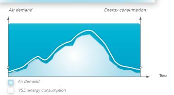
Because there is no unnecessary power generated, the Z VSD can reduce energy costs by 35% or more. Life cycle costs (LCC) of the compressor can be reduced by an average of 22%. In general, the extra cost of a VSD compressor compared to a fixed speed one can be earned back after just one to two years.
