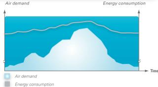
Traditional compressors working with a full load, no load control operate between two set pressure points. When maximum pressure is reached the compressor goes off load. During periods of medium to low air demand, the no load power consumption can be excessive – wasting large amounts of energy.
