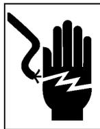
This product **must** be grounded. Grounding reduces the risk of electrical shock by providing an escape wire for the electrical current if short circuit occurs.
